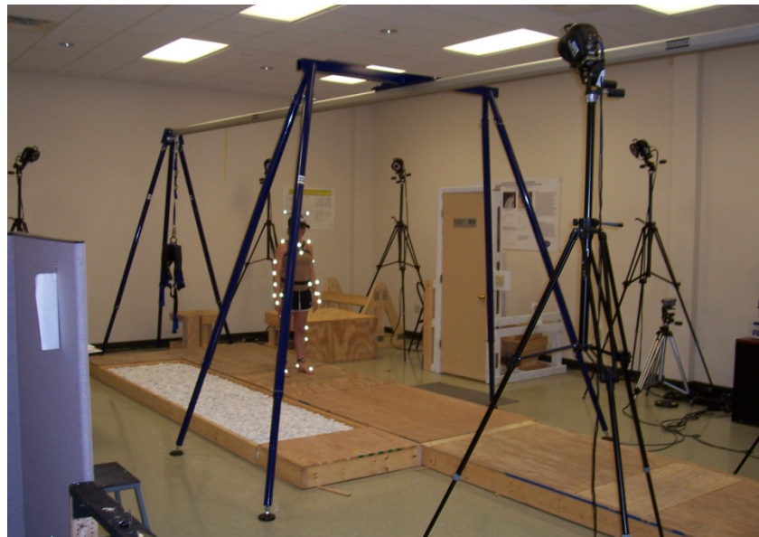
Figure 8: Configuration of Vicon Cameras for Study
